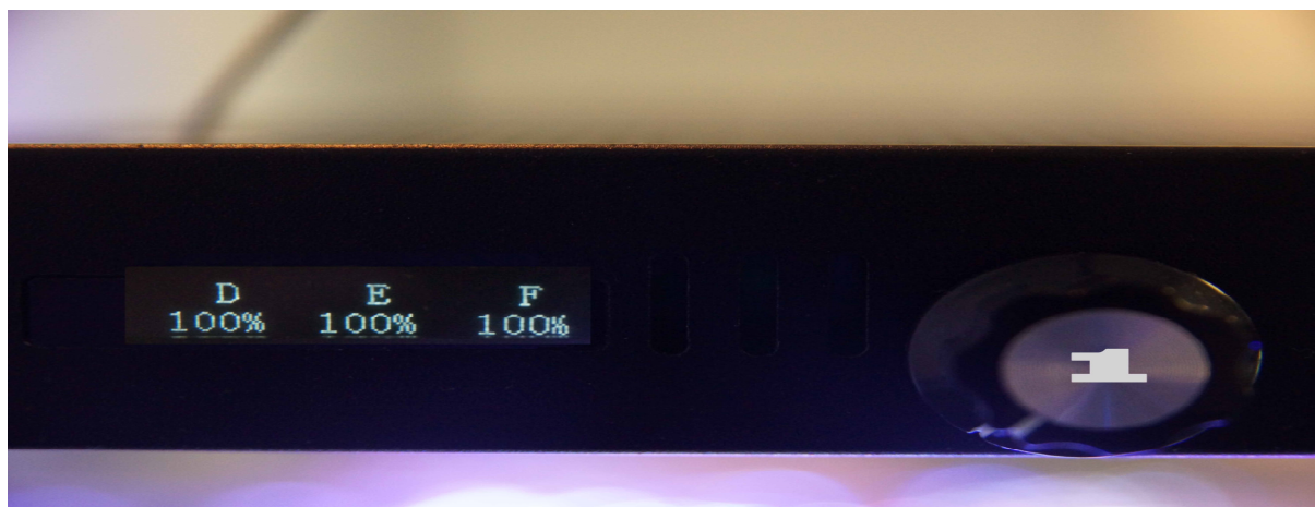
Pict. 7: By pressing the adjusting button, the individual channels are selected and they can be changed by turning the adjusting button. If you keep the button pressed for a bit longer, the manual mode is left again.
