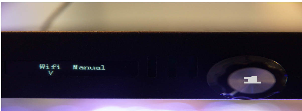
Pict. 4: By turning the adjusting button (1) you can switch between Wi-Fi and manual.
