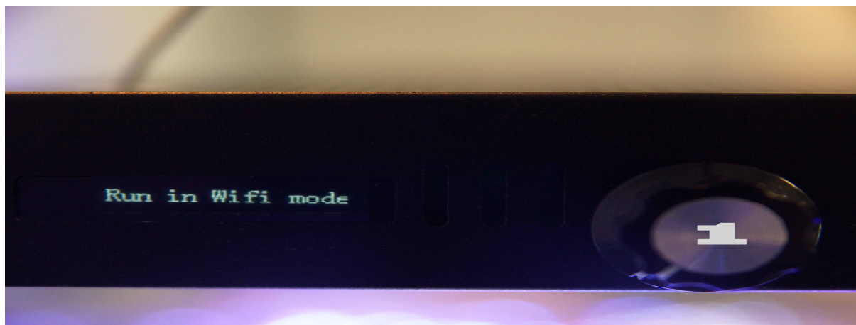
Pict. 5: After briefly pressing the button (1) "Run in Wifi mode" will appear. Now, the lamp can be controlled and adjusted via app. By pressing (1) again, you will return to the selection mode between Wi-Fi and manual.
