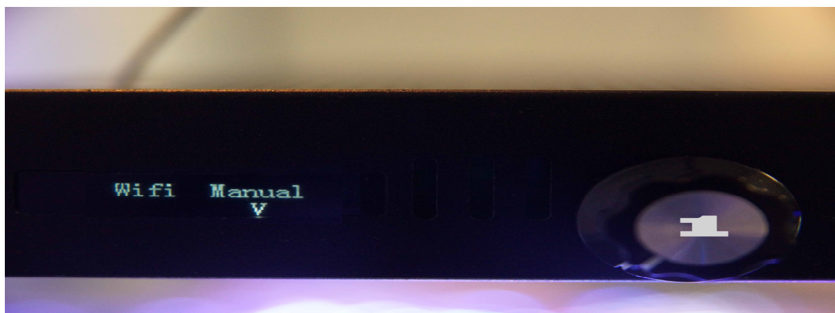
Pict. 6: If you select „Manual“ and press the adjusting button (1), you will reach the manual setting.
